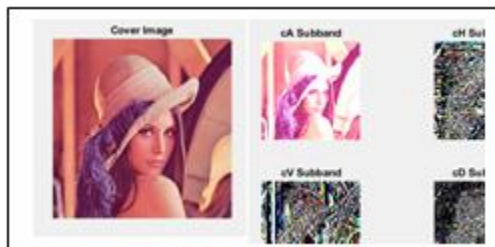
Fig. 6. Decomposition of the cover image using DWT
